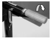
2. Move gear shift lever quickly and firmly from neutral to forward.
