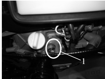
1.oil level check window
